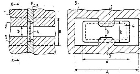
holes. The placement of the varactor in such a manner reduces the interference caused by the varactor in the interresonator coupling. A new apparatus for positioning the varactor within the resonator hole is disclosed and basically includes a conductive rod which at its top end receives the varactor.
